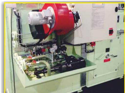
Roto Pump feeding dirty oil for incineration
